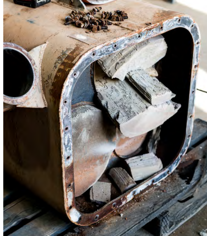
A Clogged Up DPF
